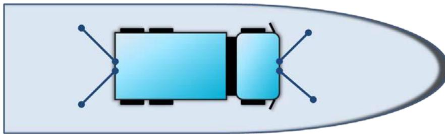
2 lashings at each end for vehicles stowed in fore and aft direction
