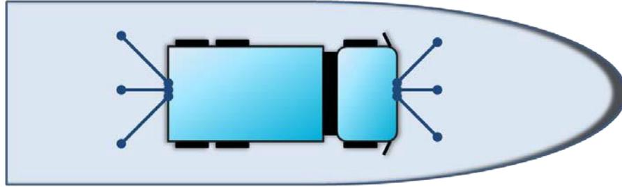
3 lashings at each end for vehicles stowed in fore and aft direction
