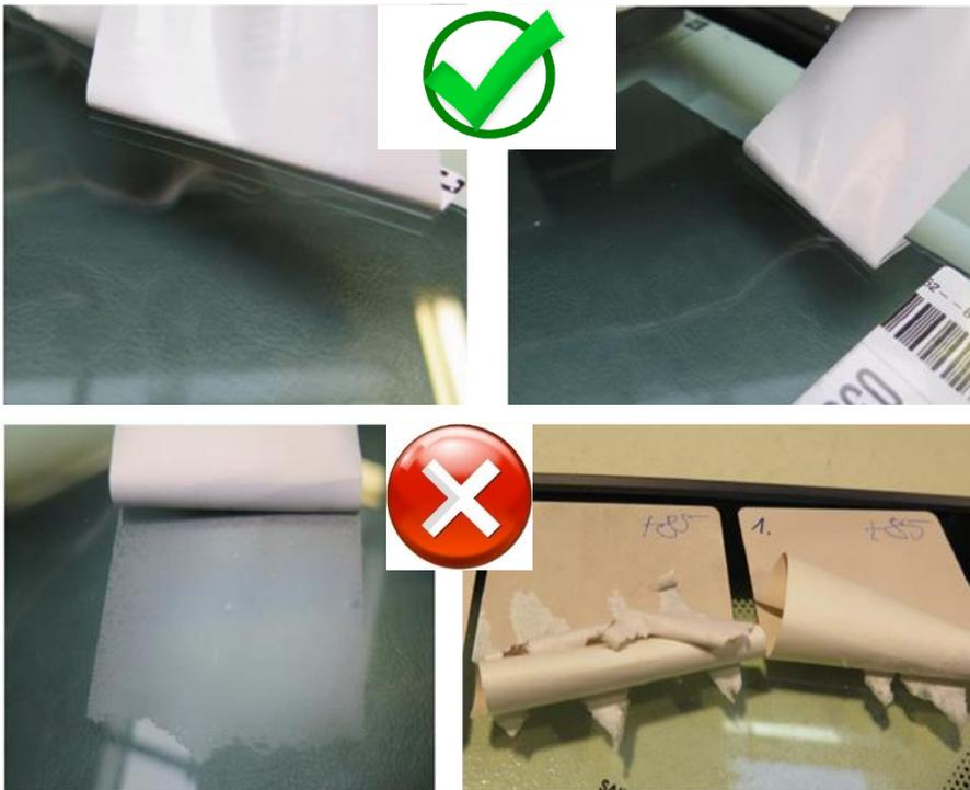
Afterwards, the labels were affixed to the window glass for 50 cycles of closing and opening of the window.
