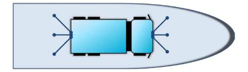
3 lashings at each end for vehicles stowed in fore and aft direction
